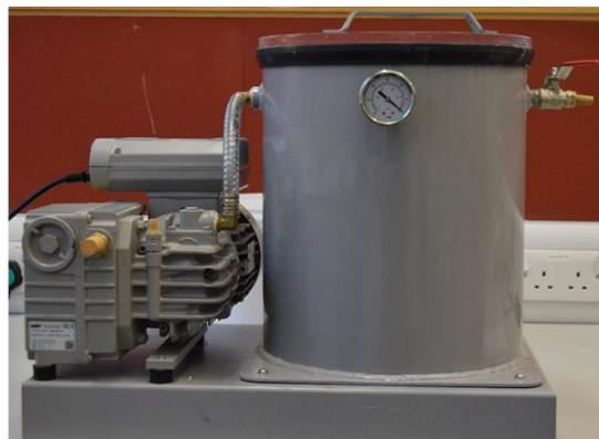
*Degassing chamber, used to remove air bubbles*
