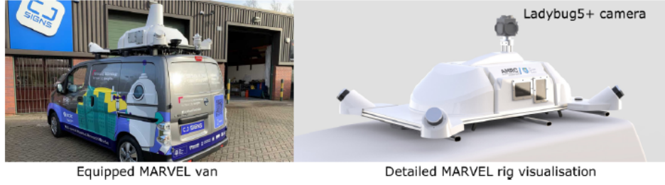
Figure 6.2: The MARVEL. This data-capturing system is used for collecting street view images for Barnsley, Doncaster and Merthyr Tydfil in this thesis. Detailed design of this data capturing system can be found in Meyers et al. [91], Dai et al. [92]
