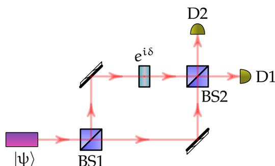
Figure 6.1: The standard two beam splitters arrangement in Mach-Zehnder interferometer. [1]
